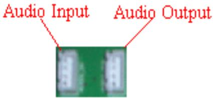
and the “CD-Audio In” or “Aux Audio In” socket on your sound card or motherboard: Also the sound card’s “Recording Control” should select the “CD-Player” or “Aux” port:
