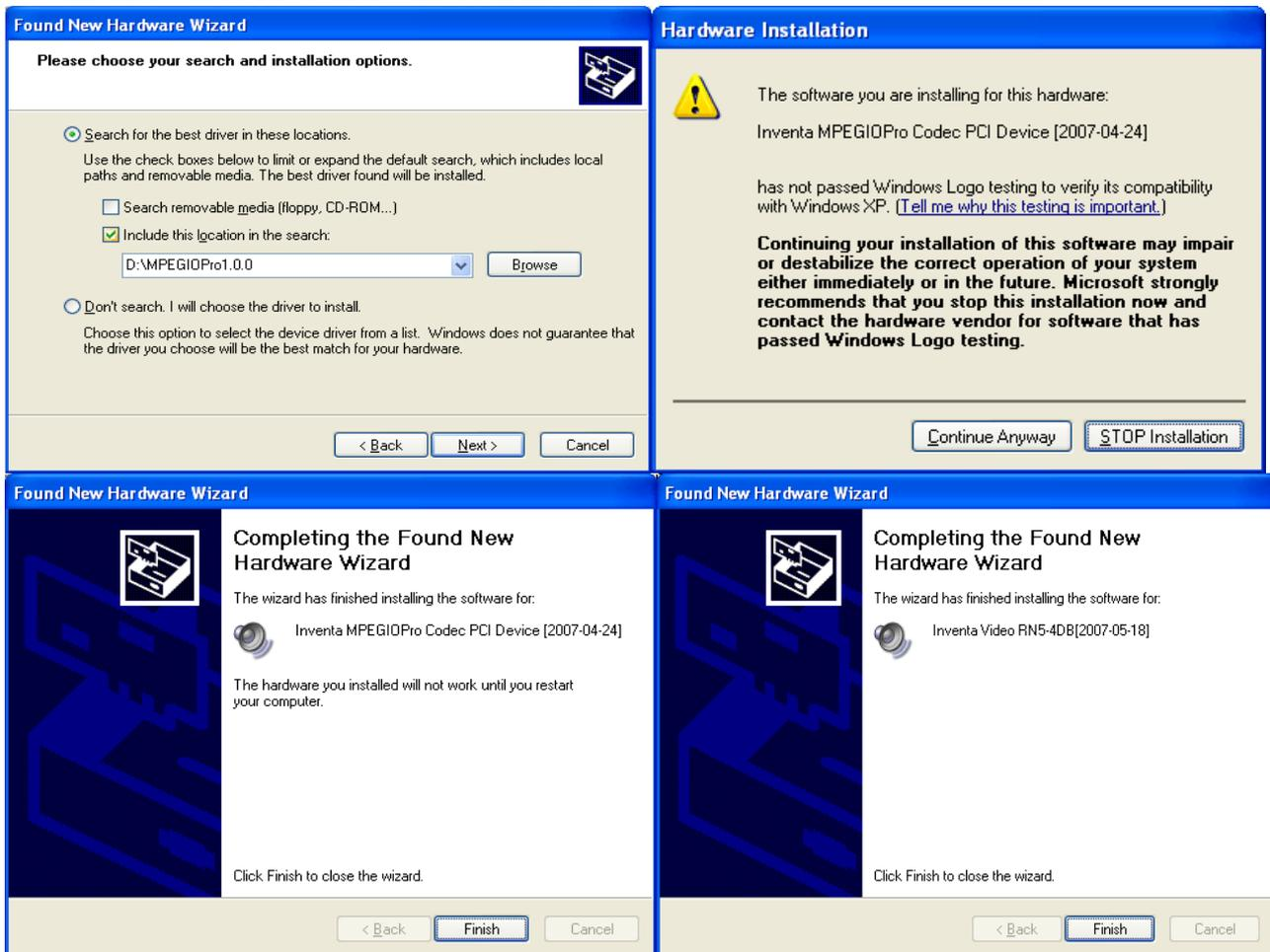
After installation of the device drivers, check the Windows' ControlPanel->System->Hardware->DeviceManager ->Sound, video and game controllers category to make sure both device drivers are listed there without question mark or exclamation mark(note each input video channel has one pair of device driver entry so one MPEGIOPro card has 8 driver entries altogether. When more than one MPEGIOPro cards are installed these entry numbers will equal to the MPEGIOPro card number multiplied by 8).
