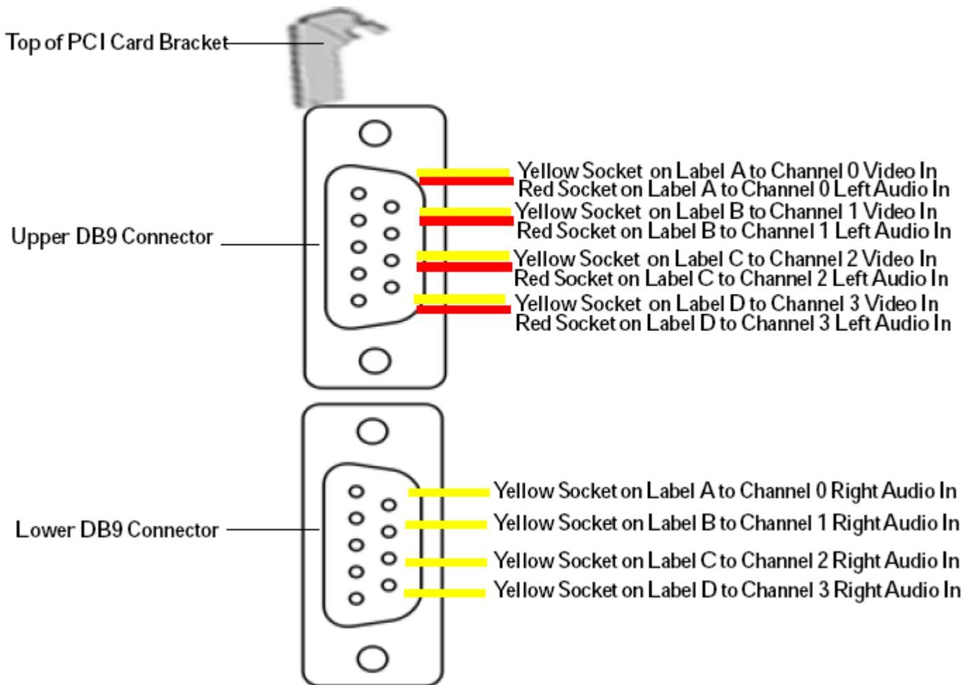
To preview (hear) live audio pass-through using PC's sound card, plug the 4-wire Audio Cable
